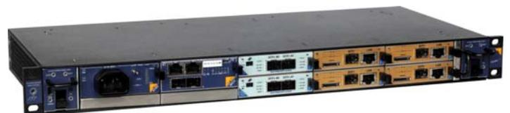
Compact TORNADO-MTCA® DSP/FPGA modular system with two T/AX-DSFPX network AMC-modules and four TORNADO-A6678® DSP/FPGA M/S AMC-modules in 19" 1U 6-slot MicroTCA® chassis with 10GbE backplane switch
