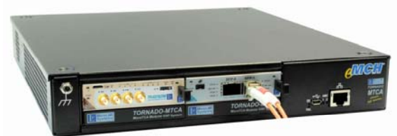
Mini TORNADO-mMTCA® DSP/FPGA modular system with TORNADO-A6678/FMC DSP/FPGA/FMC M/S AMC-module and TAX-DSPX network AMC-module in dual-slot MicroTCA® mini chassis with passive backplane
