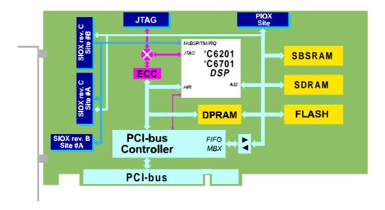
*TORNADO-P62/P67* are ultra-high performance DSP platforms with flexible modular construction for real-time DSP and data acquisition for both PCI plug-in and stand-alone applications.
