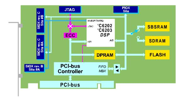
*TORNADO-P6202/P6203* are ultra-high performance DSP platforms with flexible modular construction for real-time DSP and data acquisition for both PCI plug-in and stand-alone applications.
