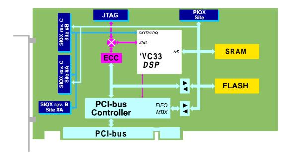
*TORNADO-P33* is high performance DSP platform with flexible modular construction for real-time DSP and data acquisition for both PCI plug-in and stand-alone applications.
