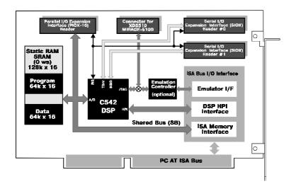
TORNADO-542L is a high performance and multifunctional DSP platform for real-time data acquisition and DSP for IBM PC ISA-bus host computers. Low cost, flexible modular system architecture and a wide selection of AD/DA/DIO expansion daughter card modules make TORNADO-542L an ideal platform for telecommunication, telephony, speech, audio, instrumentation and biomedical application as well as for OEM and education.
